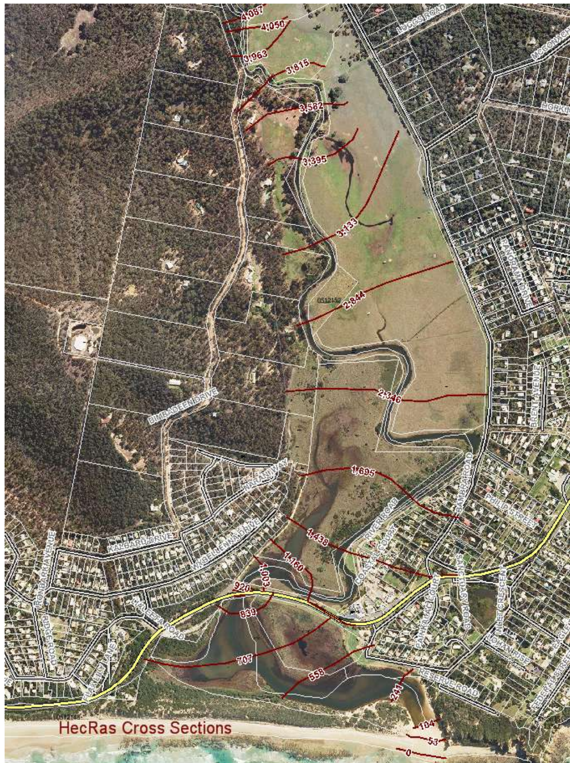
The location of the HEC-RAS cross sections are shown as red lines with their chainage in metres from the ocean.
