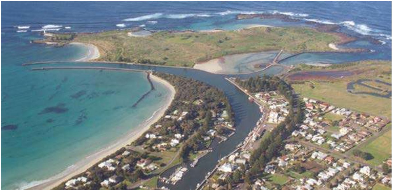
Figure 30. The Moyne River estuary mouth is considerably altered with seawalls, marinas, training walls and dredging. Photo by Peter Robertson, Warrnambool City Council.
