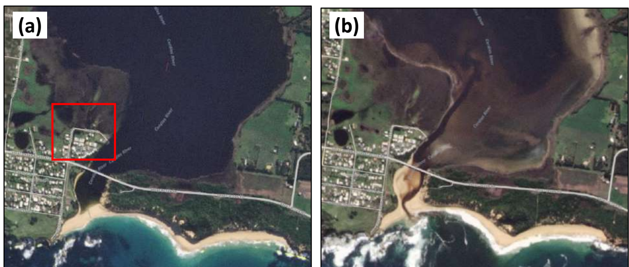
Figure 31a-b. (a) Curdies Inlet 17/06/19 showing inundation of Dorey St (red square); (b) 23/06/19 after second opening showing drainage of floodwaters. Images from Planet Team (2019).
