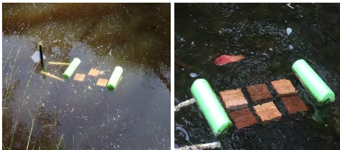
Figure 3.3. Floating experimental frame. A) Floating experimental frame attached to an anchor post with one set of blocks. B) Close-up showing two sets of wood blocks at different stages of biofilm development.
